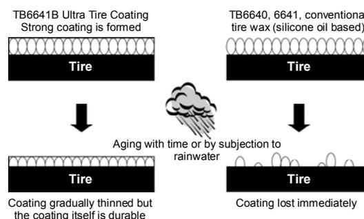
Figure 6. Comparison of weathering mechanisms to conventional TB products
