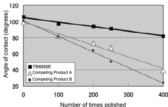
Figure 4. Durability of water repellency of TB6550E
