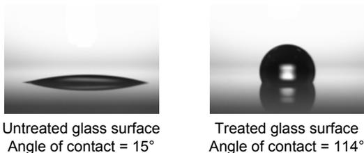
Photo 3. Water repellency of TB6550E-treated and untreated glass surface
