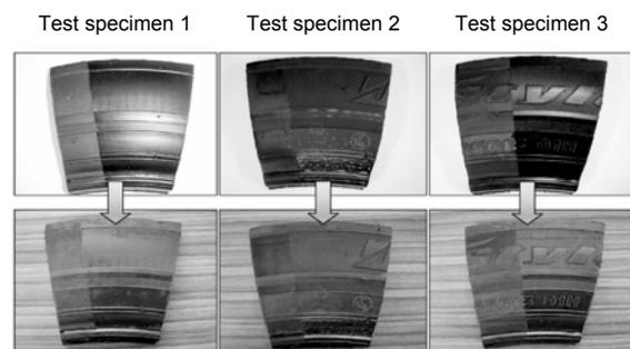
Photo 6. Surface of tire after testing with De Mattia flex tester
