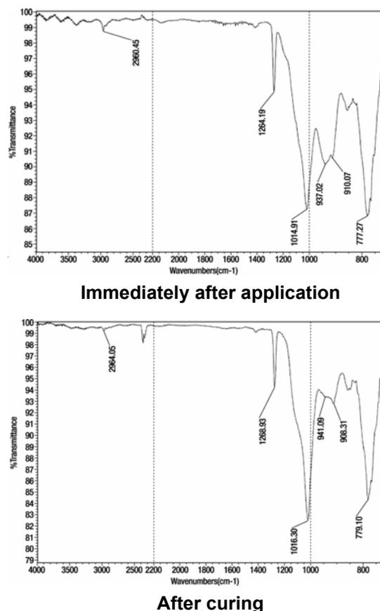
Figure 1. IR spectra of TB6644/6644B coating
