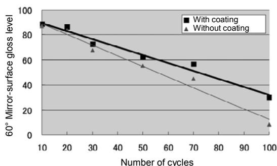
Figure 2. Results of weathering test using TB6644
