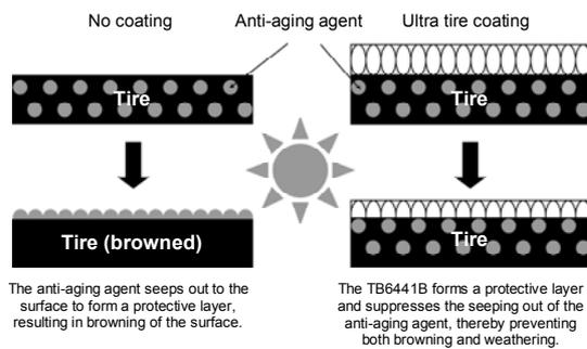
Figure 5. Mechanism of weathering prevention by TB6641B
