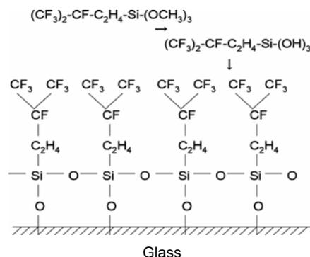
Figure 3. Schematic image of incorporation of a perfluoroalkyl silane compound onto a glass surface
