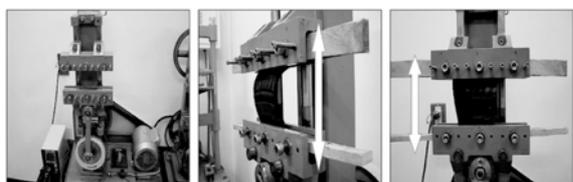
De Mattia flex tester      Beam moves vertically to bend the test specimen
