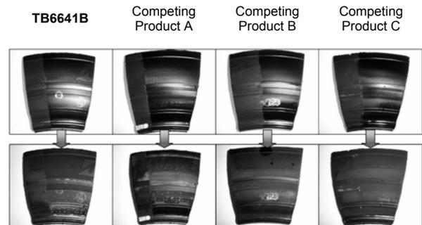
Photo 4. Tire surface after 10-day exposure under the xenon-arc-lamp weathering tester (Top: before test; bottom: after test)
