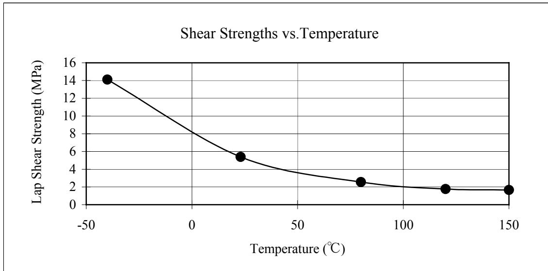
Steel (SPCC, SB) test coupons were cleaned with xylene, open time for 5 minutes, cured for 7 days at 23°C, 50% RH.
