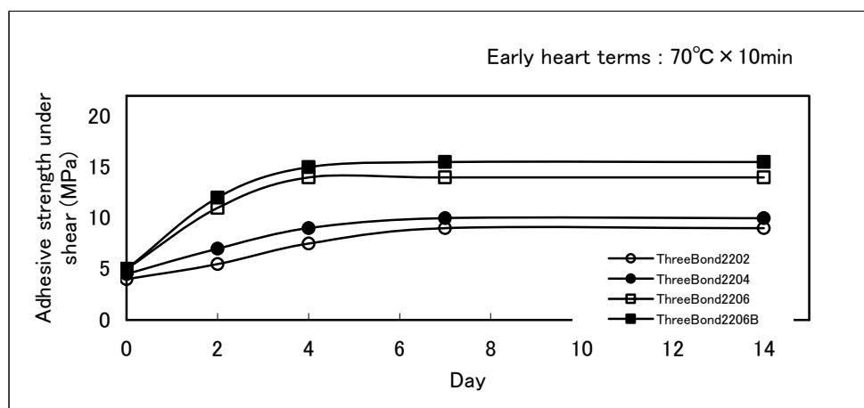
\* Iron-iron test pieces which is left at 25°C atmosphere is measured in regulation time. Trigger curing ability changes conditions a lot by the usage, material, etc. It is recommended to check the bonding conditions using actual parts and determine the optimum curing conditions.
