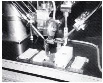
Photo 9 Example of application of sealant to motor shaft (horizontal application method)
