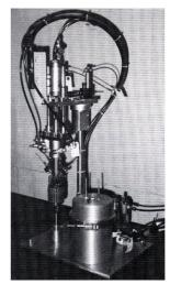
Photo 8 Example of application of sealant to motor shaft (vertical application method)
