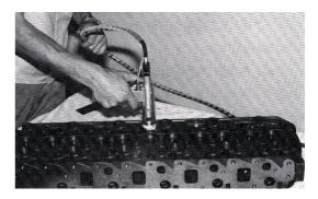
Photo 11 Example of application of sealant to inner circumference of sand draining holes of diesel engine cylinder heads (3B Coater RTM)
