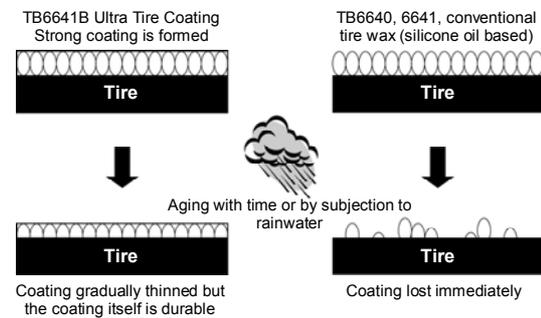
Figure 6. Comparison of weathering mechanisms to conventional TB products
