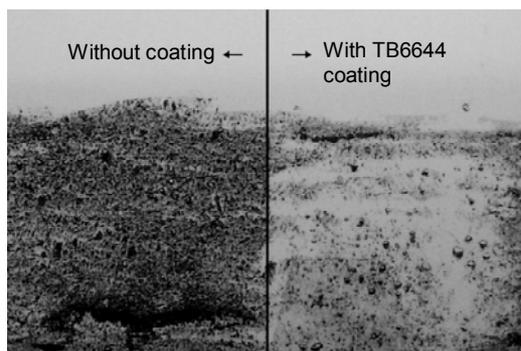
Photo 1. Results of stain prevention test using TB6644
