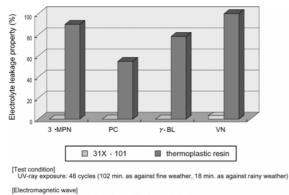
[Electromagnetic wave] 3-MPN: 3-Methoxy propionitrile, Gamma-BL: Gamma-butyrolactone, PC: Propylene carbonate, VN: Valeronitrile (I<sub>2</sub>:0.1M, KI:0.05M, MePrimi:0.6M, and TBP: 0.5M were added into them respectively)
