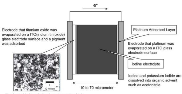
Titanium oxide layer that a pigment was adsorbed
