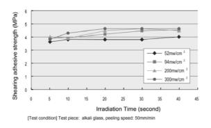
Figure 5, Relationship between irradiation time and shearing adhesive strength by UV-ray intensity
