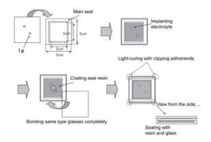
Figure 7, How to create dummy cells
