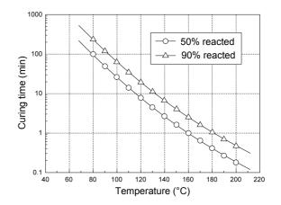
Figure 1. Curing rate of liquid epoxy resins
