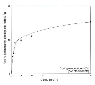
Figure 2. Curing speed of ThreeBond 3065/3096
