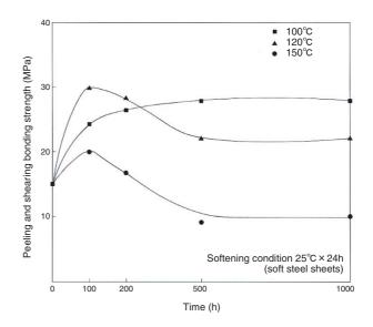
Figure 3. Heat aging of ThreeBond 3065/3096
