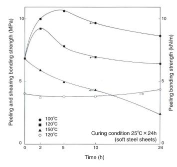
Figure 4. Heat aging of ThreeBond 1735
