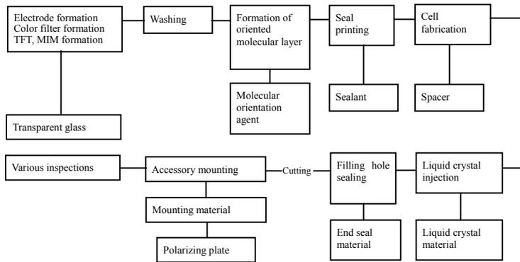
Fig. 3 General LCD production process
