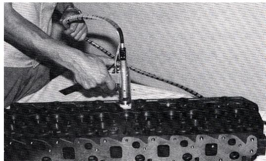
Photo 11 Example of application of sealant to inner circumference of sand draining holes of diesel engine cylinder heads (3B Coater RTM)
