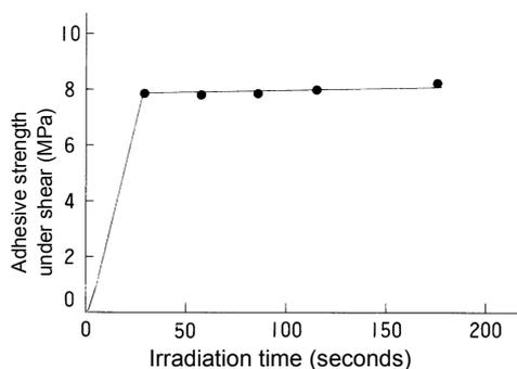
Fig. 2-1. Relationship between the irradiation time and the adhesive strength of the VL-001 type under shear for a glass/glass test piece
