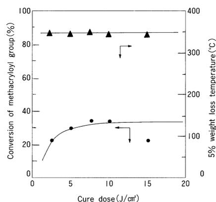
Fig.1-1. Light-polymerization and 5% weight loss temperature of 6FDAI.
