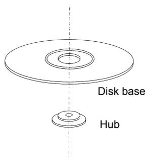
Fig. 5-1. Optical disk structure
