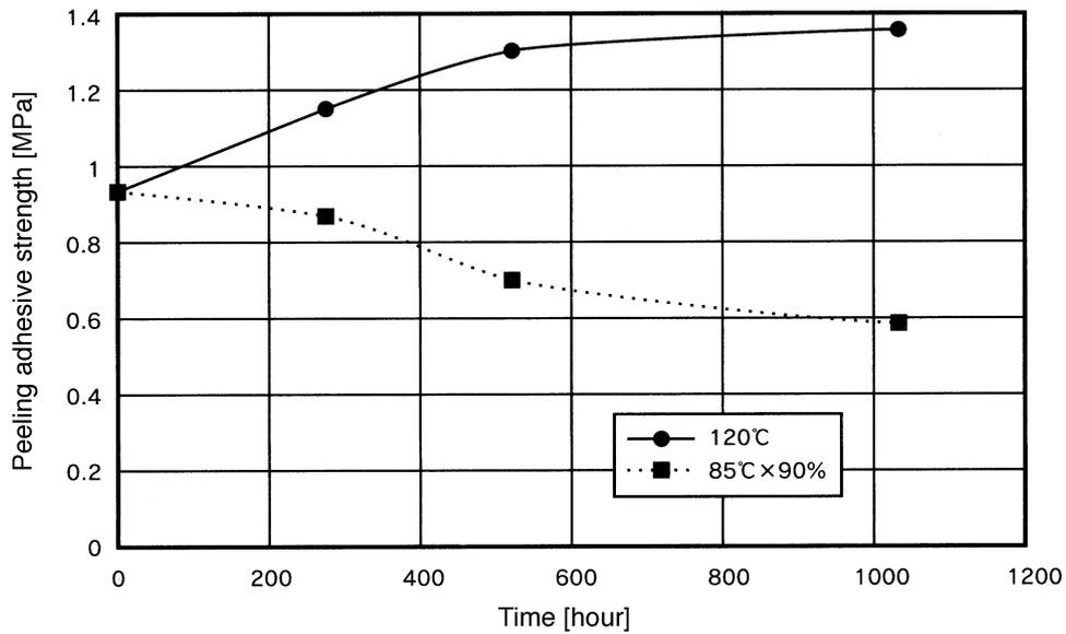
Fig. 6. Results of peeling adhesive strength test
