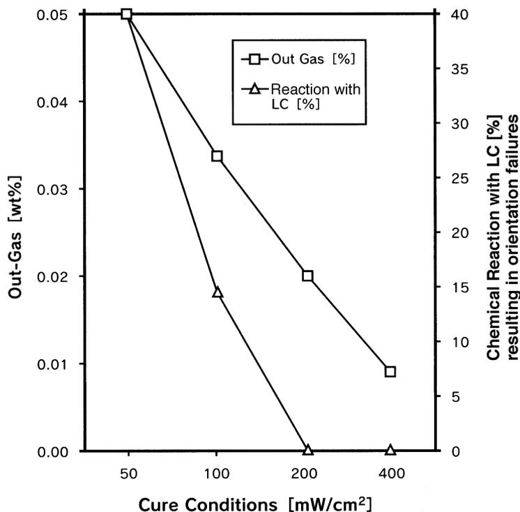
Fig. 5. Out gas and chemical reaction with LC vs. curing condition
