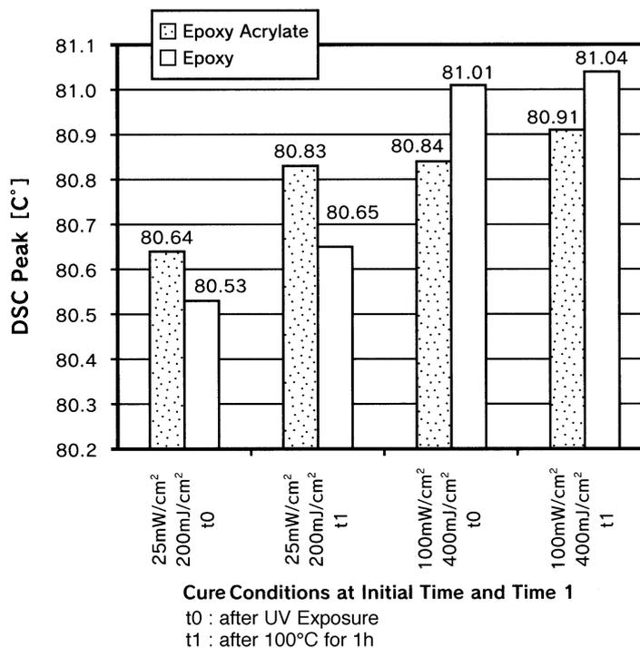
Fig. 4. DSC results for different UV-curing conditions
