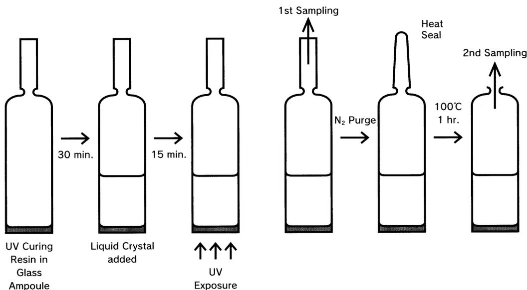
Fig. 2. Testing a base resin
