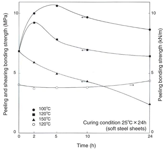
Figure 4. Heat aging of ThreeBond 1735
