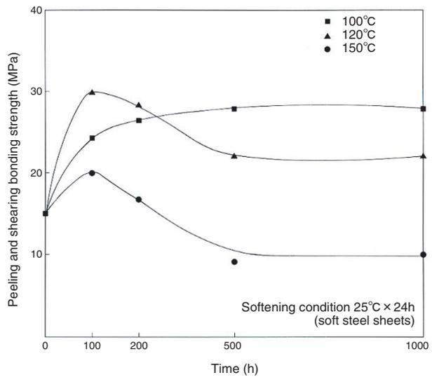
Figure 3. Heat aging of ThreeBond 3065/3096
