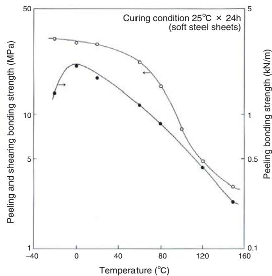
Figure 1. Temperature dependencies of bonding strength for ThreeBond 2087
