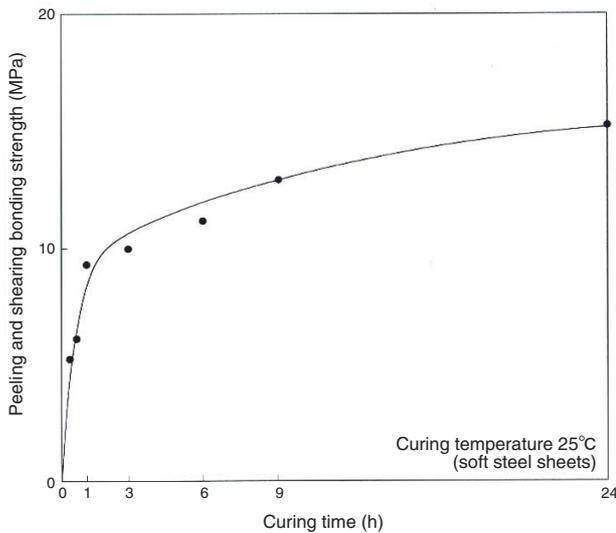
Figure 2. Curing speed of ThreeBond 3065/3096
