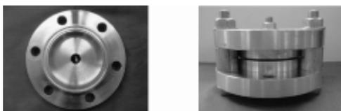
Figure 6. Flange for pressure resistance test
