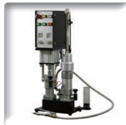
Cartridge pump (ACB-20) Pen-shaped manual open/close valve (pencil gun)
