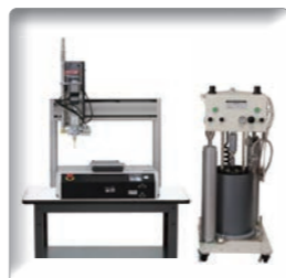
Pump for pails (PBIII) Constant-speed injection head (fixed-quantity booster) Desktop three-orthogonal-axis robot (RT7-30)
