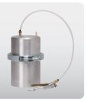
This simple dispenser enables hand-operated pencil gun application of low viscosity liquids via a pressure tank. Coating is easily adjusted via air pressure of the tank and opening or closing of the pencil gun lever. Replacing materials is also simple.
